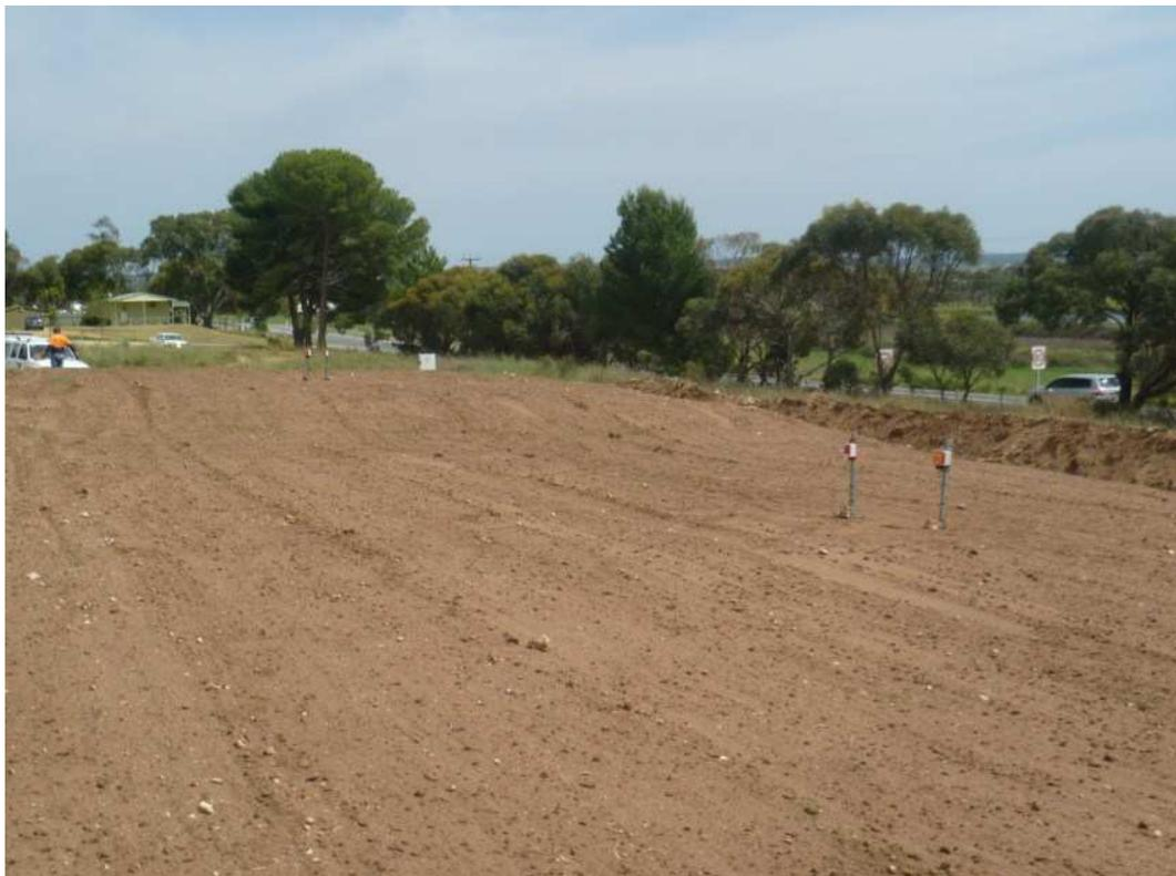
\* High profile and 2 soil moisture sensors in background and sensors on low profile in foreground.
