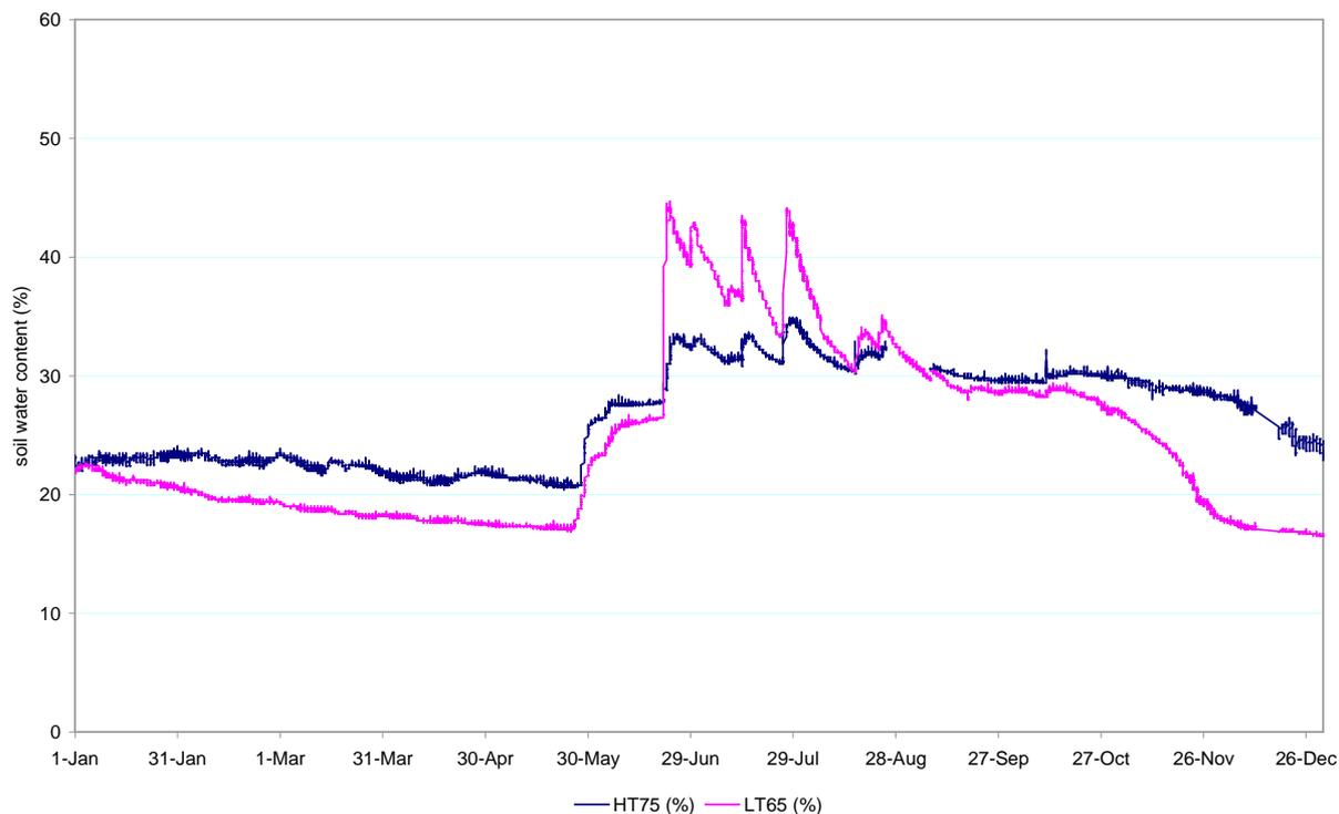
**Figure 11: Soil Water Content above the Underlying Plastic Liner**
