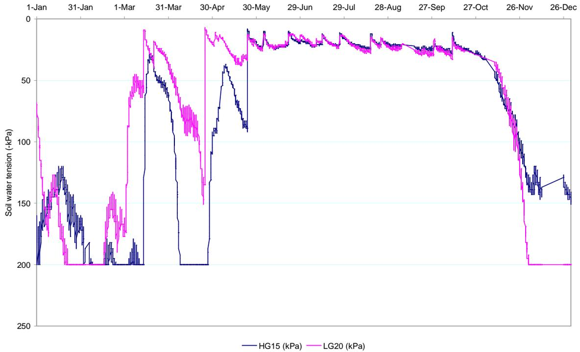
**Figure 12: Soil Water Tension at 200mm below the surface**
