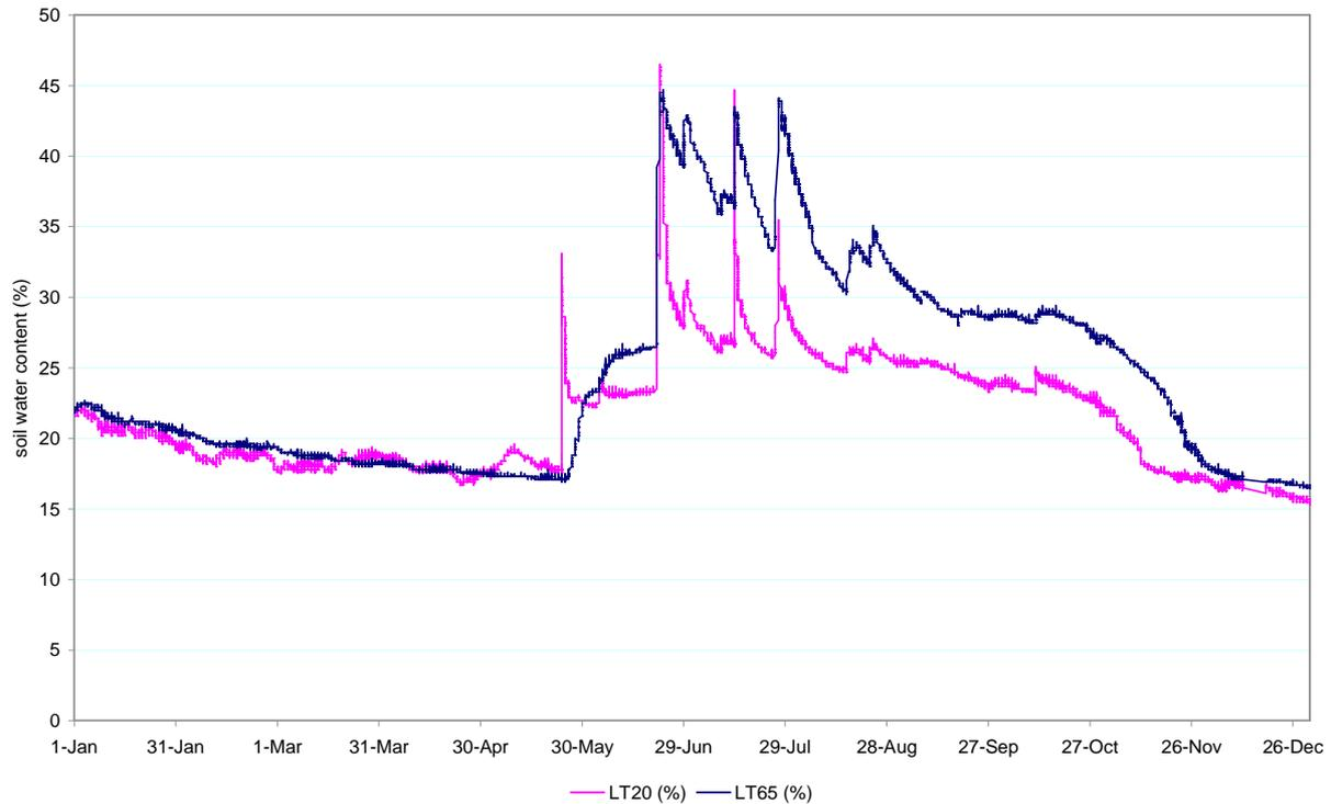
**Figure 9: Soil Water Content through the Low Profile Soil Layers**
