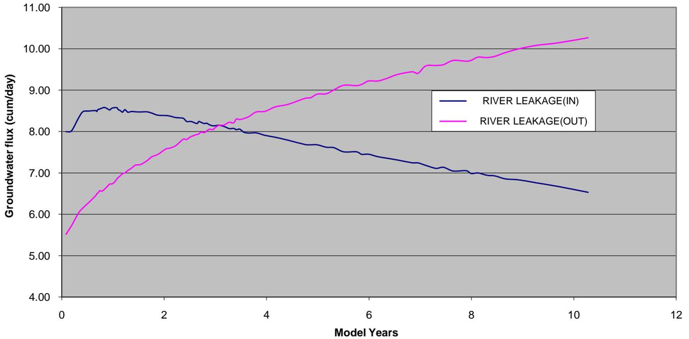
RIVER LEAKAGE (IN) represents flow from the model river calls into the shallow aquifer.
