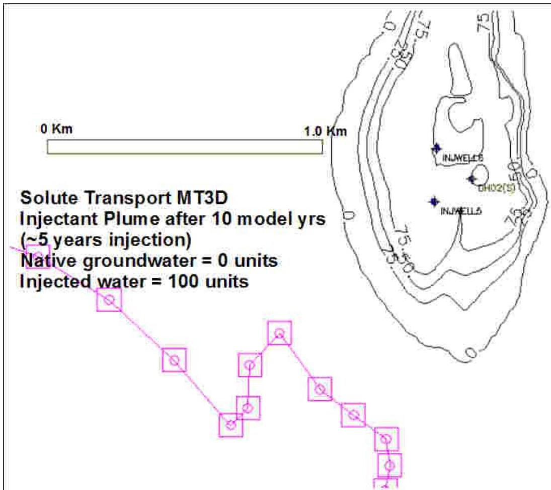
**Figure 8: MT3D Model Plume of Injected Water after 10 years Model Time (Approx 5 years Injection)**
