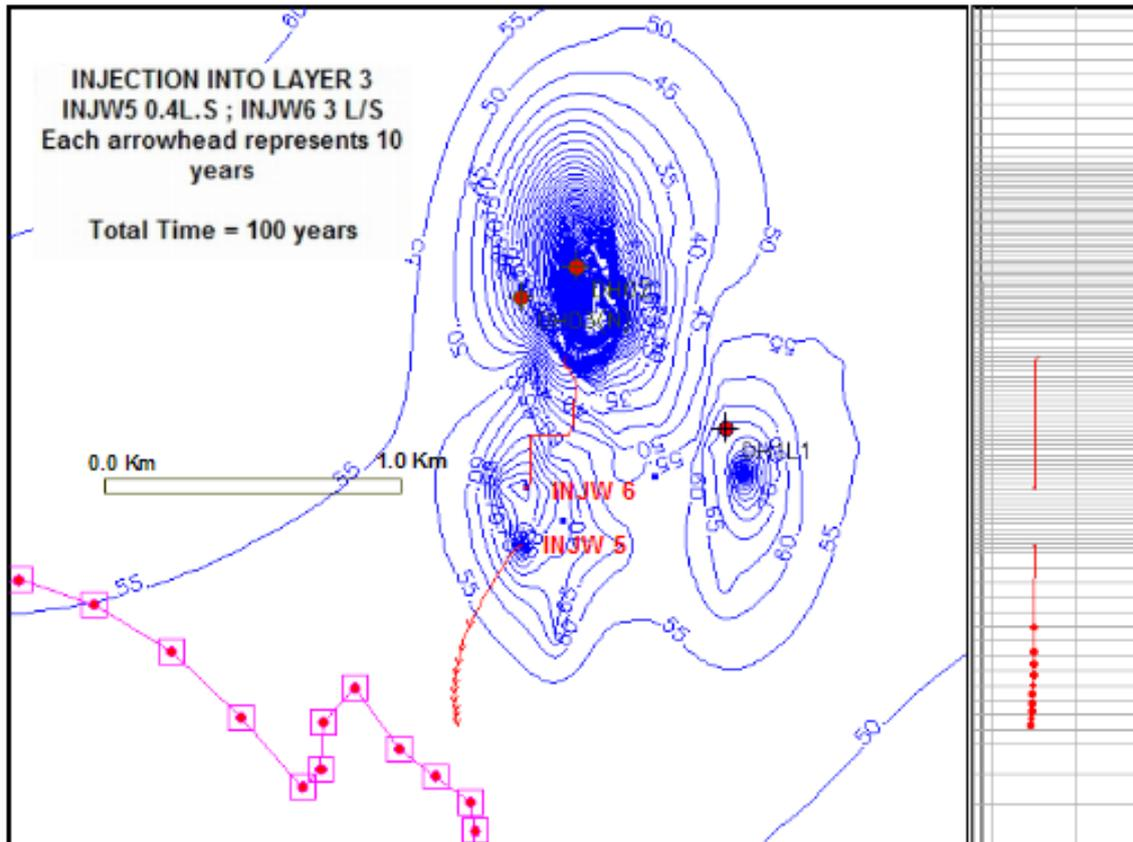
**Figure 7: Model Heads after 10 years with flow paths from new injection wells**
