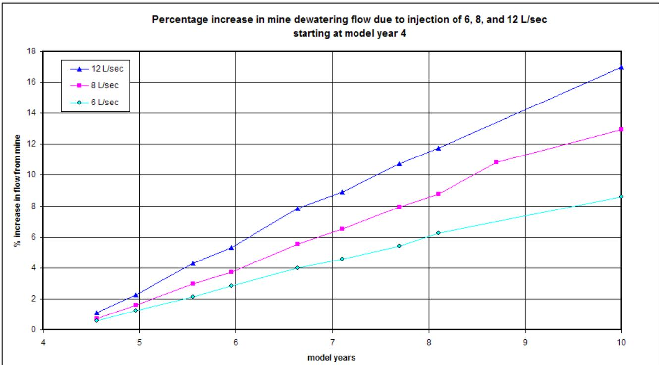
Figure 3 Percent increase in predicted minewater flow due to injection
