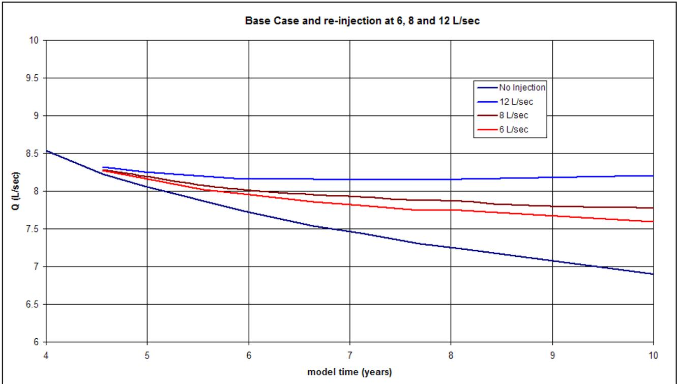
Figure 2 Model-predicted minewater flows in response to injection
