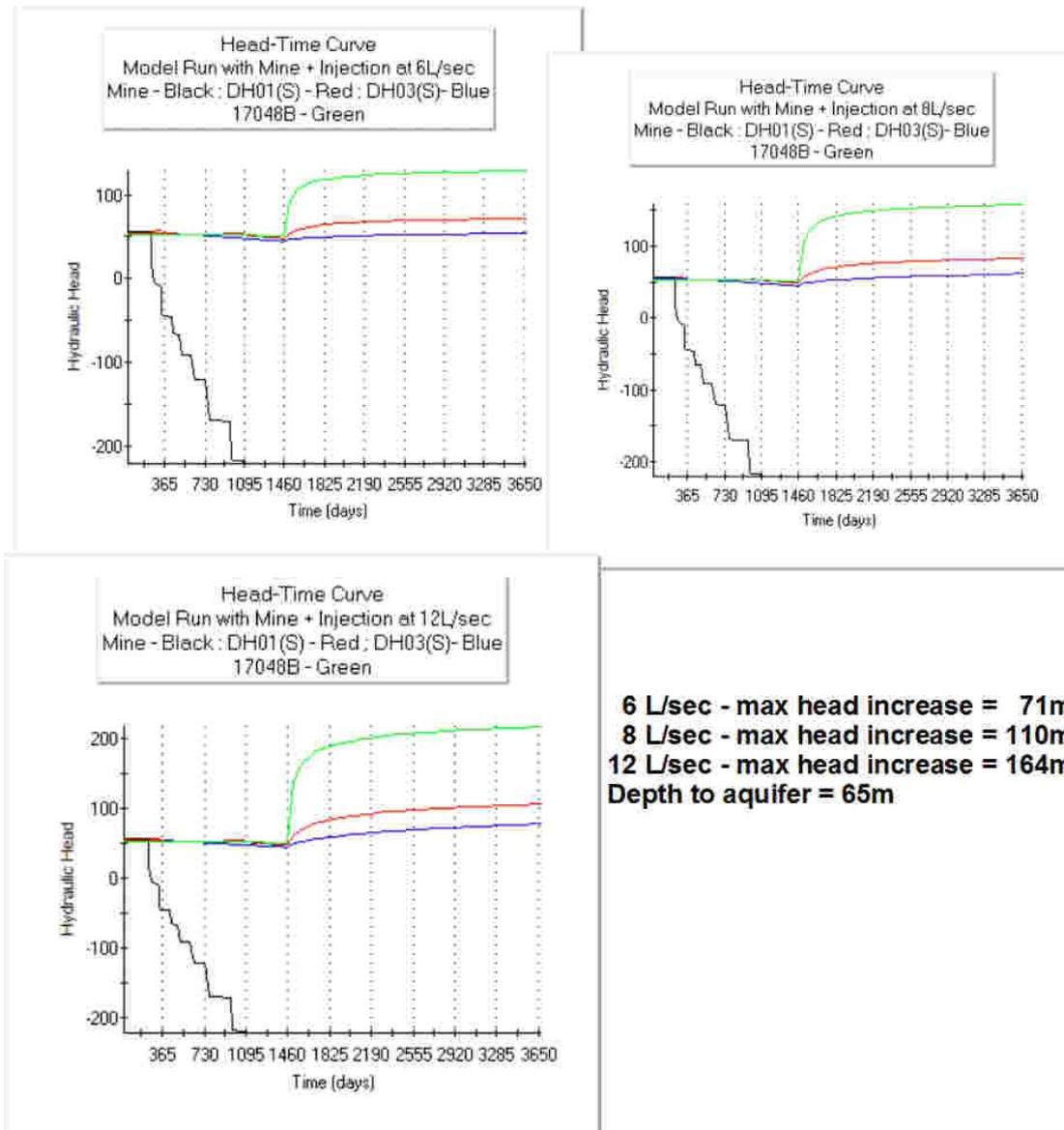
**Figure 4 Heads vs time for injection at 6, 8 and 12 L/s**
