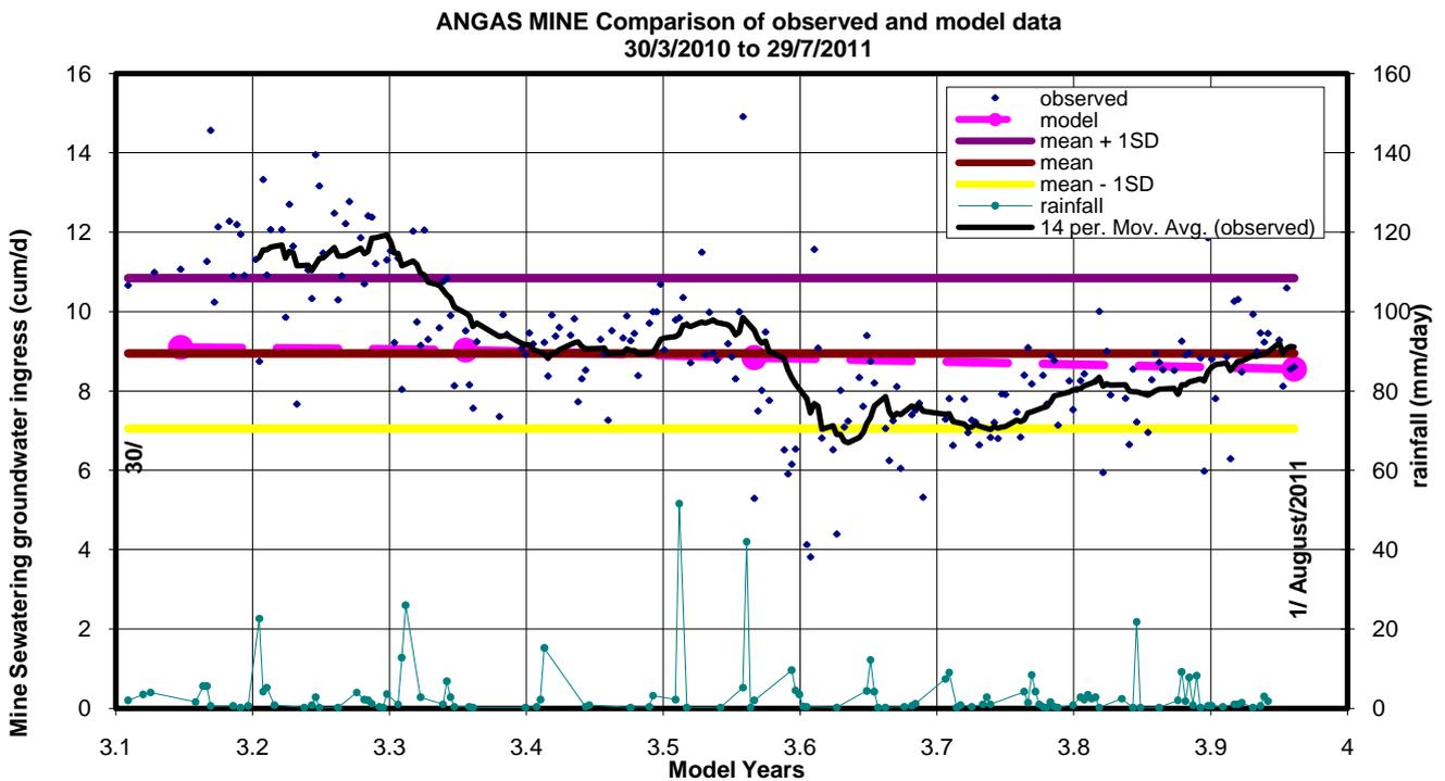
**Figure 1 Comparison of Measured and Model predicted Minewater Discharge**
