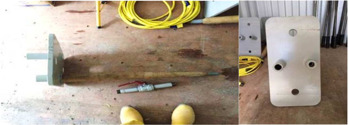
Plate 1: Spear-Shaped, Jumbo-Installed, Malleable Rubber, Borehole Packer
