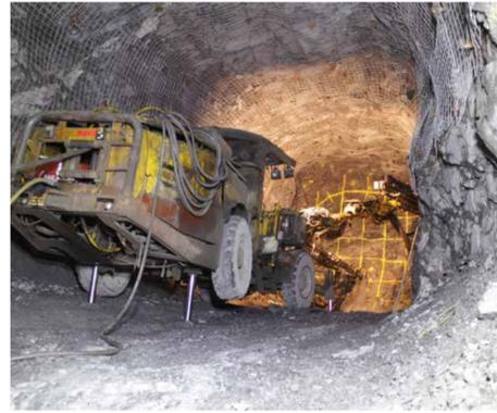
A 'Jumbo' drill rig drilling out a development face in a decline tunnel
