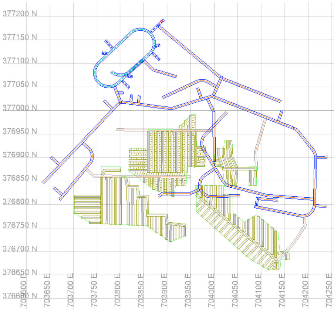
Figure 9: Typical flitch extraction concept.
