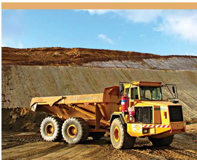
40 tonne Volvo dump trucks haul waste rock and ore to the surface via the Rankine Decline at the Angas Zinc Mine.
