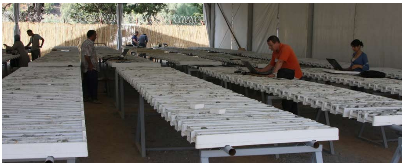
Geologists undertake drill core logging at the Tala Hamza exploration facility, Algeria.
