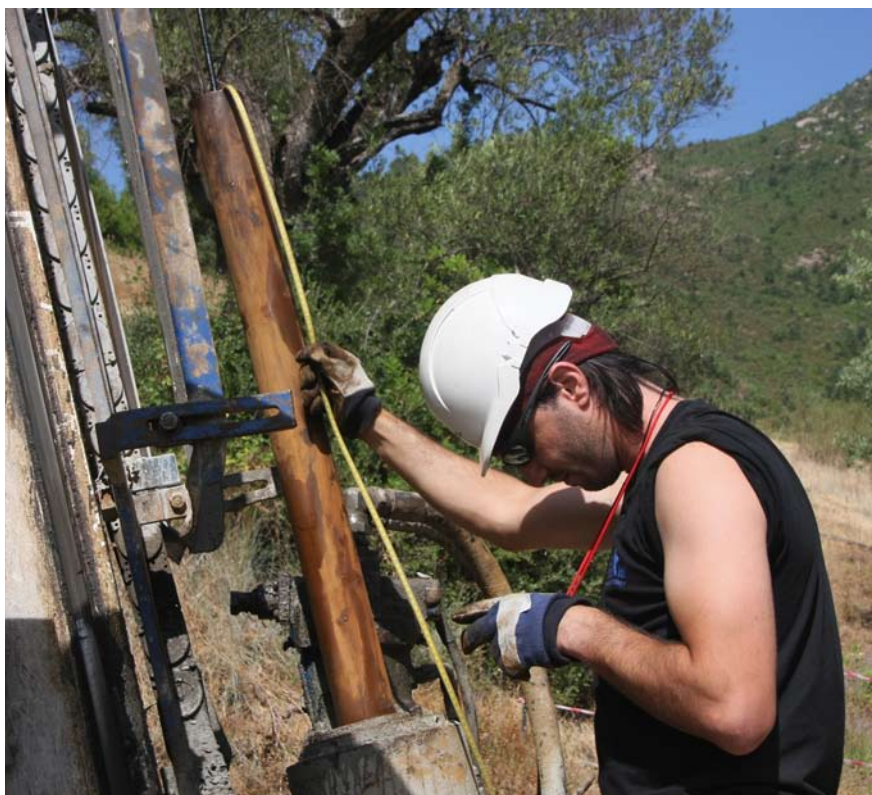
Hydrogeological testing in a diamond drill hole at Tala Hamza, Algeria.
